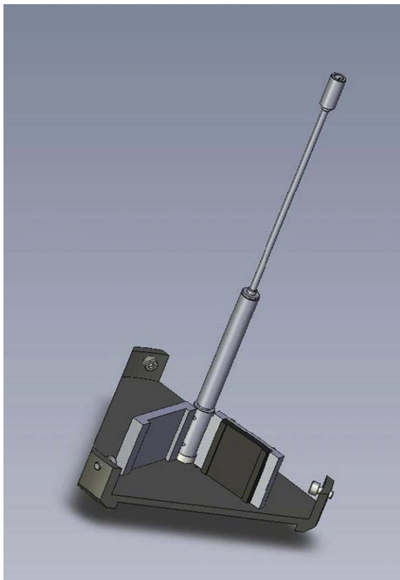
Fig. 1. Scheme of the plates used for deposition and removal of a-C:H films.
